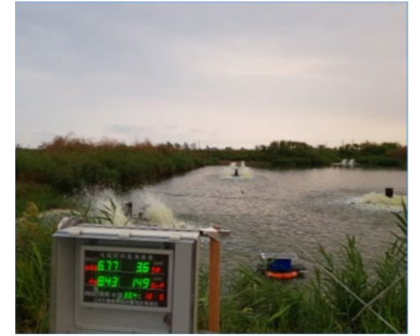
Real-time water monitoring system
